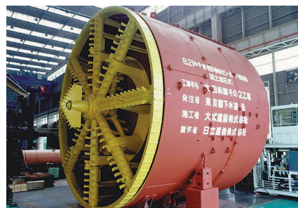
▲ Second-phase construction of the Ohta main sewerage tunnel by the Tokyo metropolitan government (Diameter: 8.21 m)
