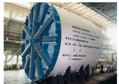
▲ Metropolitan expressway, Central Loop Shinjuku Line (outer line) by the Metropolitan Eexpressway Public Corporation (Diameter :12.02 m)
