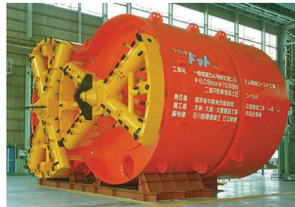
▲ DOT shield tunneling in the Rijo section of the Hiroshima Astram line (new transportation system)
