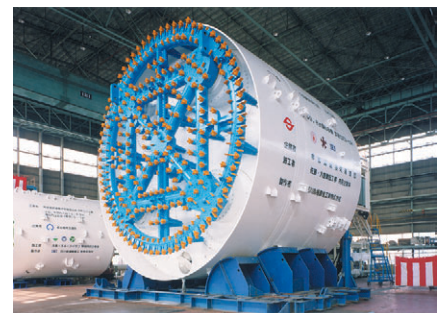
▲ Construction in the Honjo work section of Teito Rapid Transit Authority subway line No.11 in Tokyo (Diameter: 9.6 m)
