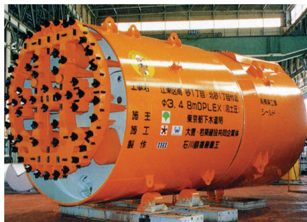
▲ Re-construction at Minamisuna 1 chome and Kitasuna 1 chome in Tokyo (Diameter: 3.48 m)
