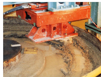
Test of mortar excavation by spike bits
