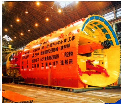
Extruding Concrete Lining Method
