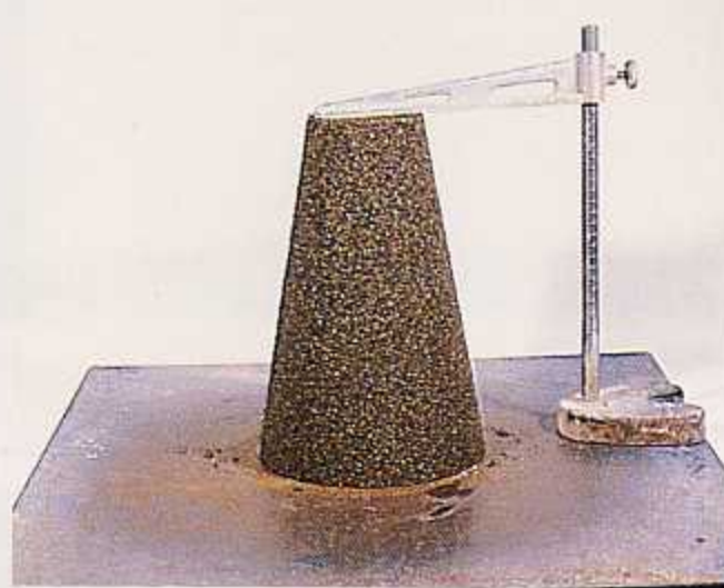
Discharged Excavated Soil Slump Test
