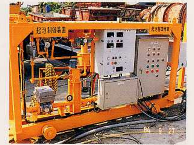
Foam Control System Car
