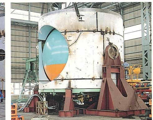
組立中 Main shield (with sphere inside)
