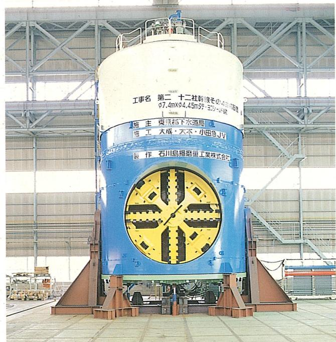
Test assembly in the factory
