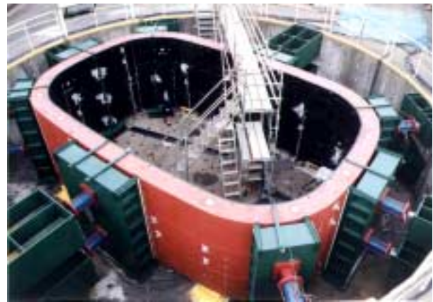
Figure 10. Loading test on composite segment rings.
