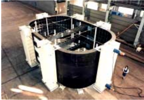
Figure 11. Loading test on DC segment rings.
